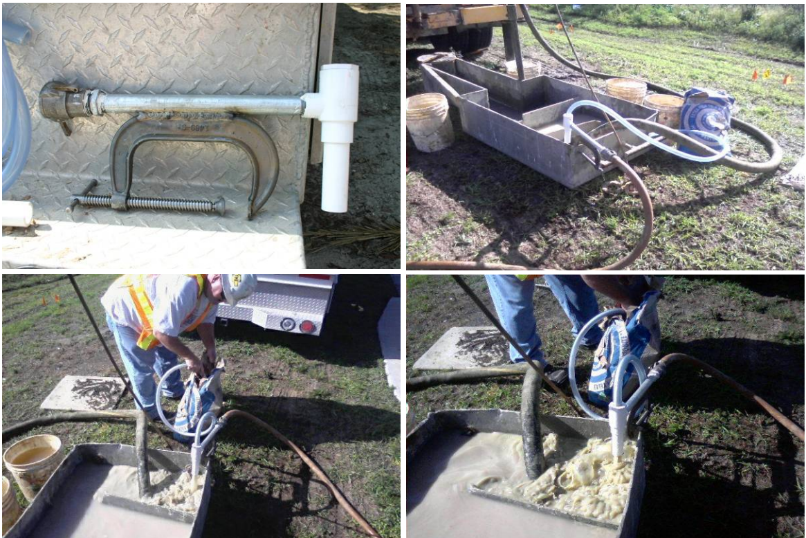
Figure 4.17. Single eductor unit mounted to drill rig slurry pan.
