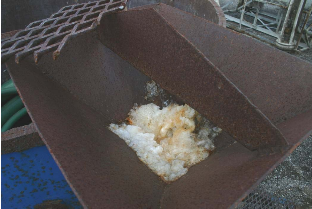
Figure 2.9. Polymer gel build-up in throat of venturi hopper.
