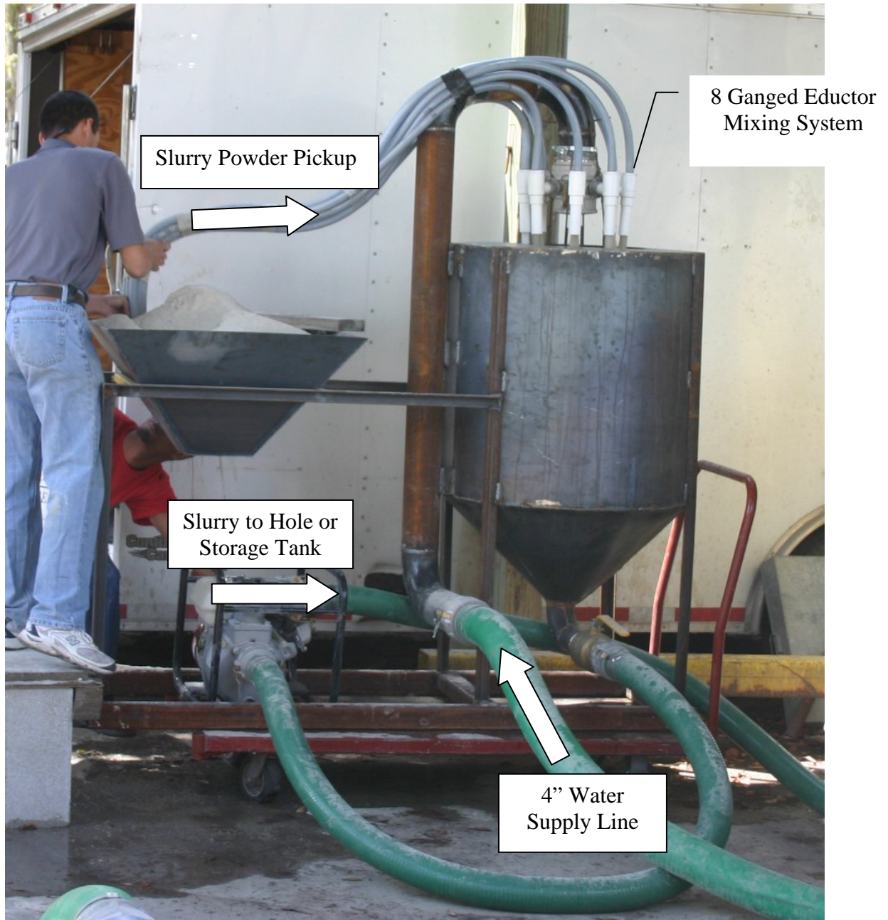
Figure 4.15. Multi-gang eductor system.
