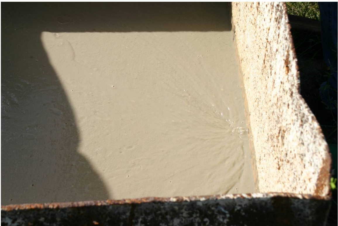
Figure 4.25. Initial slurry mixture with 8 eductors.
