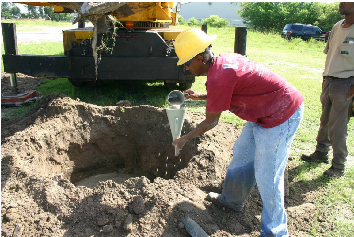
Figure 4.27. Viscosity testing at excavation.
