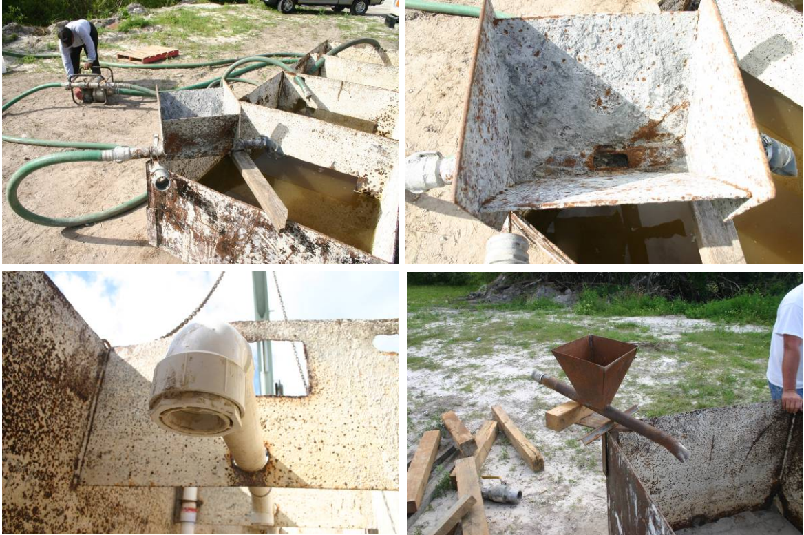
Figure 2.10. 1600 gallon slurry mixing tank (top left), venturi hopper (top right), tank recirculation / agitation system (bottom left), and alternate venturi hopper (bottom right), Courtesy of R.W. Harris, Inc..
