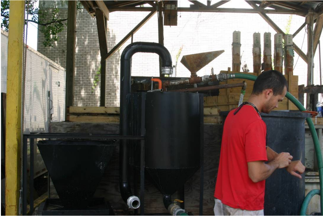
Figure 3.29. High shear pump with venturi hopper plumbed into funnel-bottom recirculating tank.
