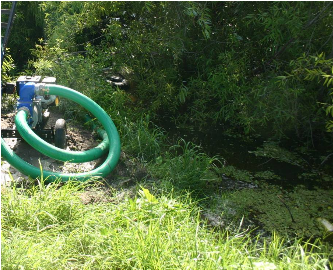
Figure 4.23. Water supply pump drawing from pond with filter box.
