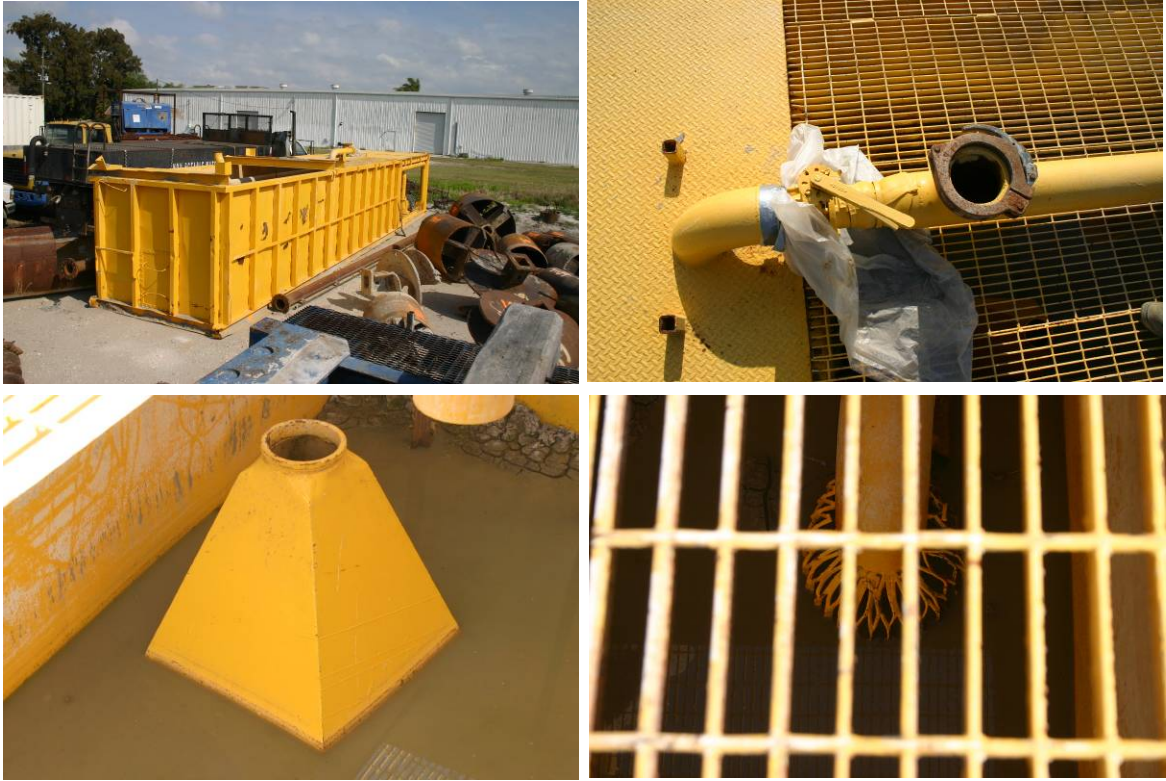
Figure 2.12. 9500 gallon slurry mixing tank (top left), venturi port (top right), removable hopper (bottom left), and re-circulation pump pick-up near bottom of tank (bottom right), Courtesy of Case Atlantic, Inc..
