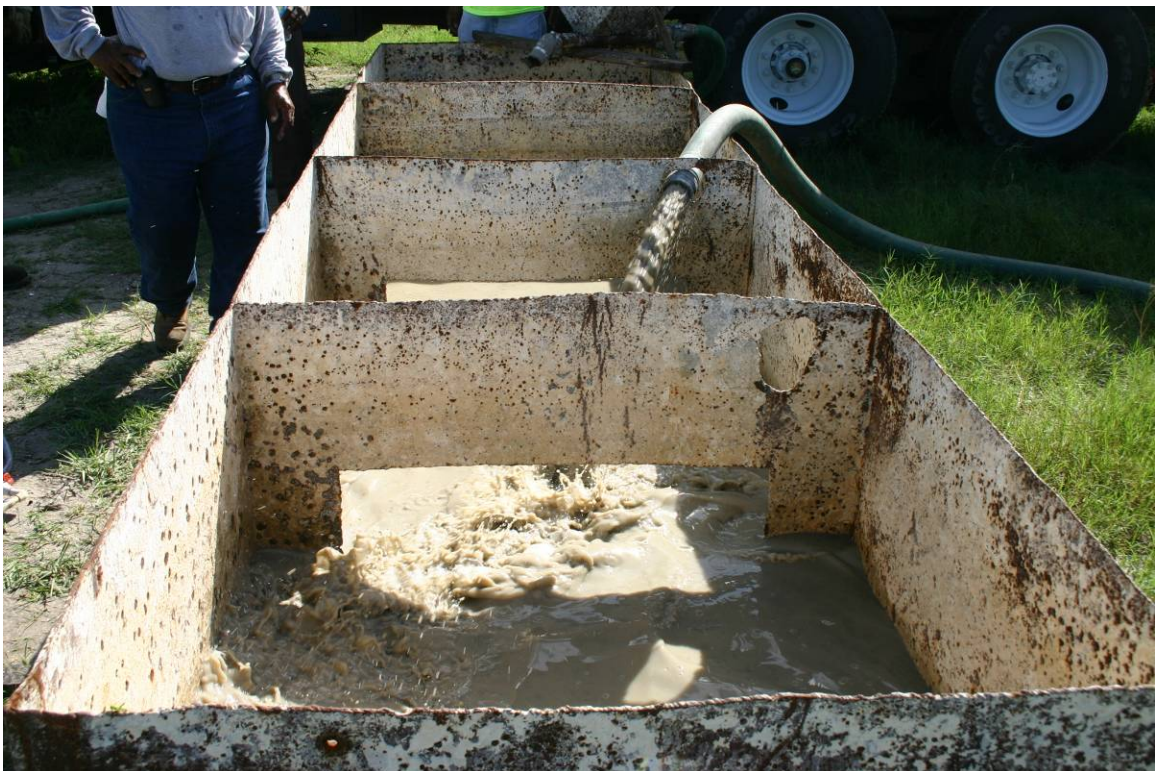
Figure 4.21. Slurry moved to 1600 gallon recirculating tank.
