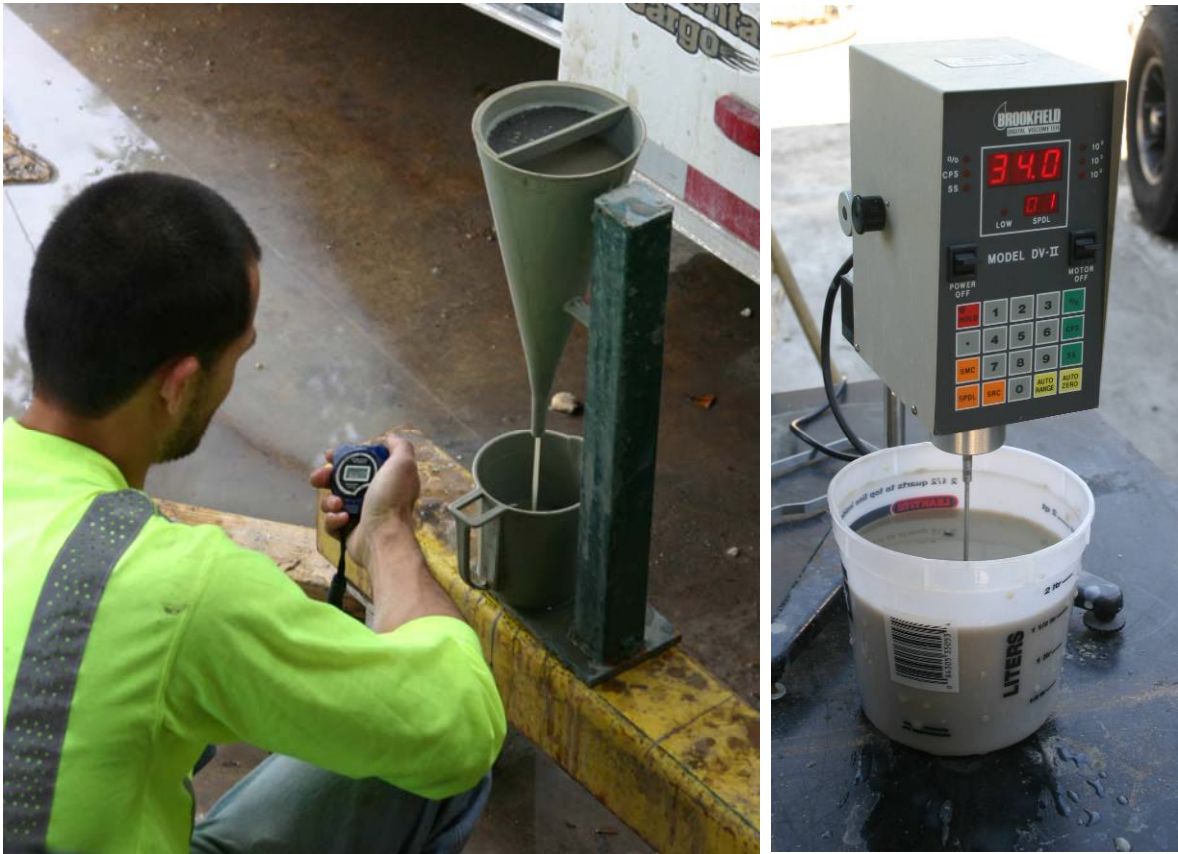
Figure 3.21 Manual (left) and automatic (right) viscosity measurements used in the study.
