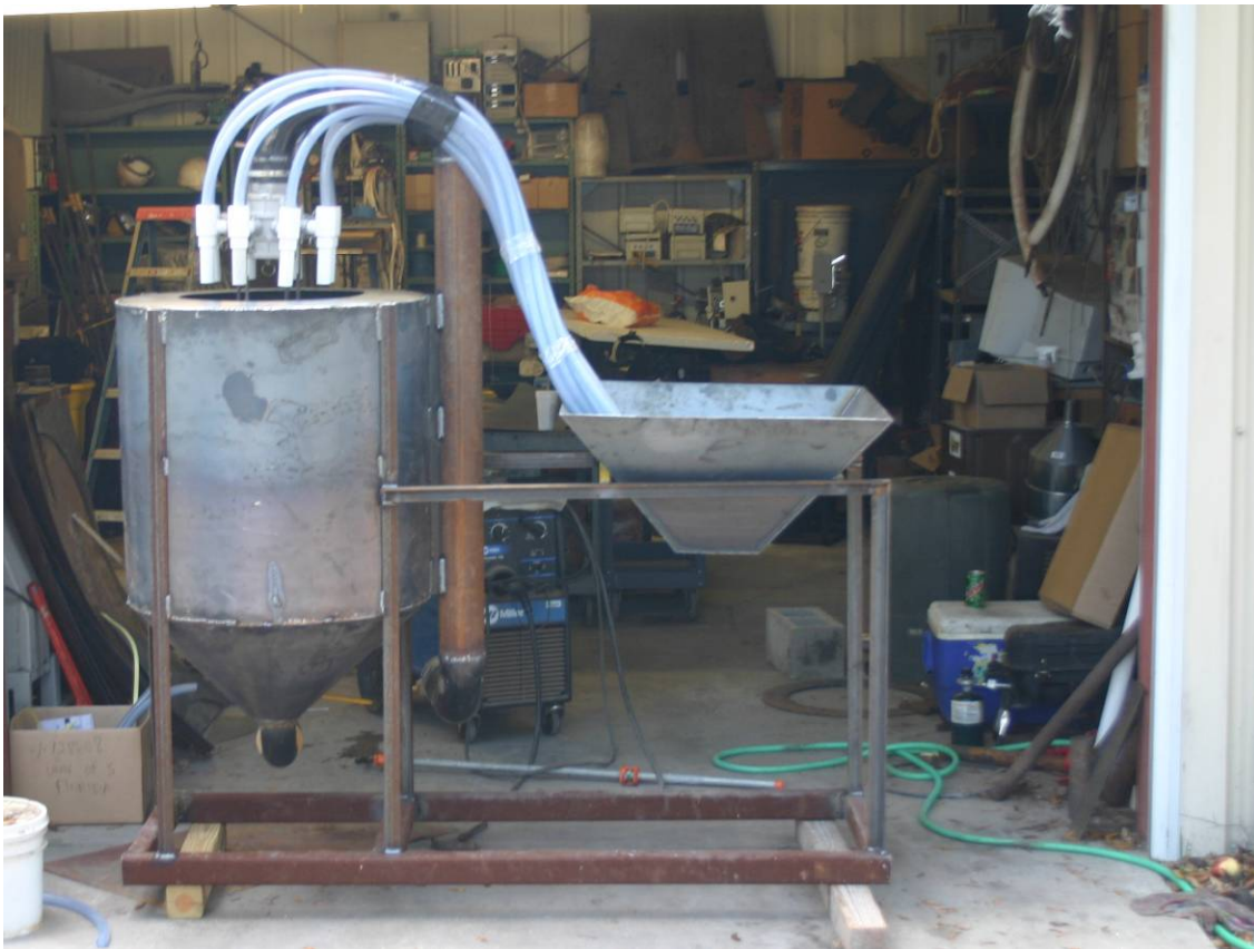
Figure 4.18. Multi-gang eductor mixing system sent for field implementation.
