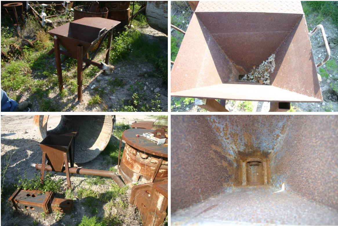
Figure 2.13. Venturi hopper with breaking table (top left), residual clumps of mineral slurry (top right), venturi hopper with extended discharge pipe (bottom left), and nozzle welded into supply line at base of hopper (bottom right), Courtesy of Case Atlantic, Inc.
