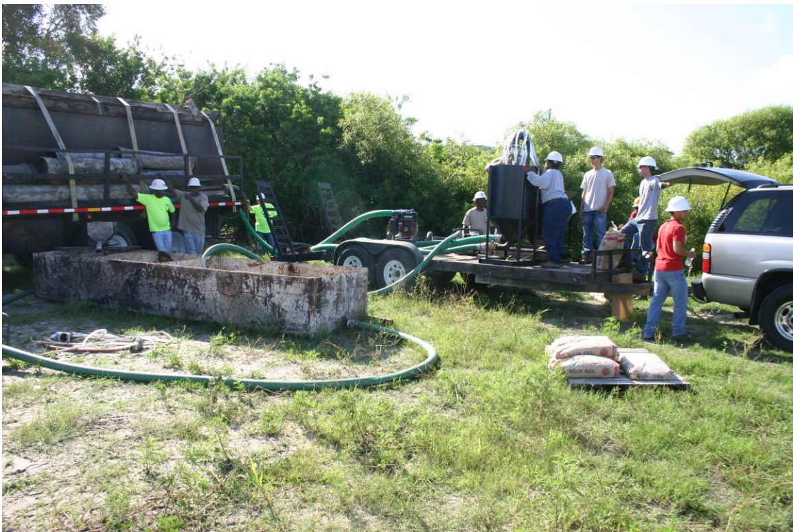
Figure 4.19. Overview of setup at R.W. Harris yard with water truck, 1600 gallon holding tank, and multi-gang eductor system.
