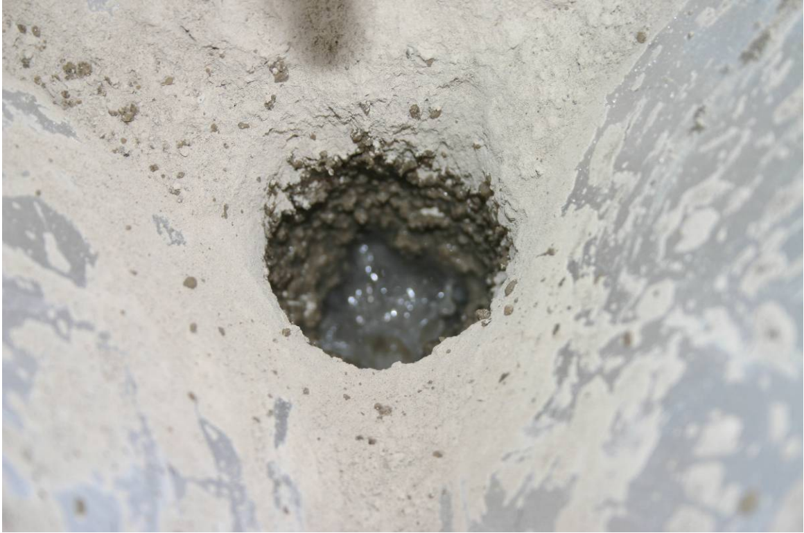
Figure 2.8. Bentonite build-up in throat of venturi hopper.
