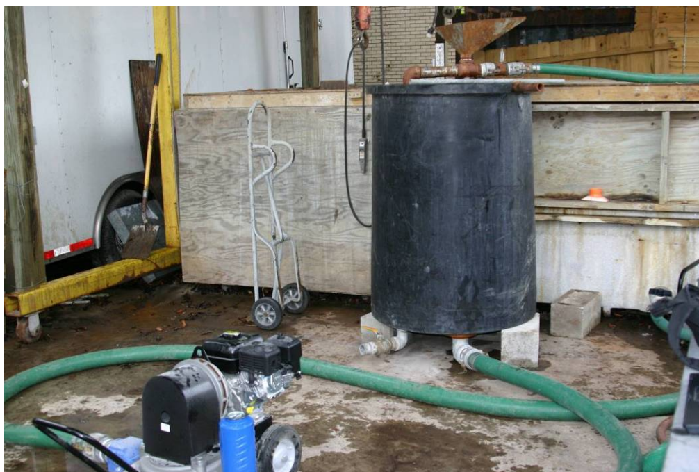
Figure 3.23. Initial plumbing of diaphragm pump and venturi hopper.
