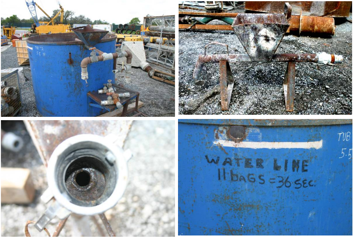
Figure 2.11. 1100 gallon slurry mixing tank (top left), venturi hopper (top right), reduction tube / nozzle (bottom left), and field mix guidelines (bottom right), Courtesy of Coastal Caisson, Inc.
